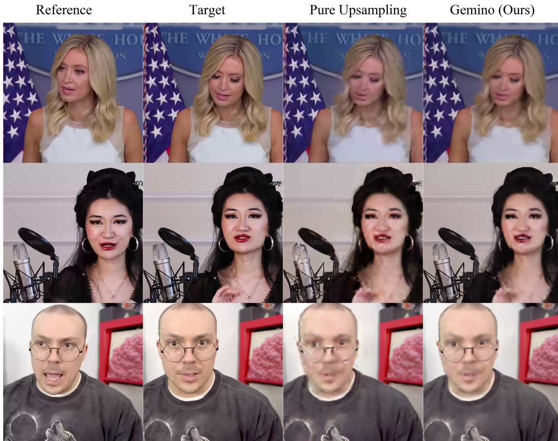
Figure 3-9: Visual comparison across different model architectures. Compared to Gemino, Pure upsampling misses the high-frequency details of the microphone (row 2) and lends block-based artifacts on the face (row 3).
